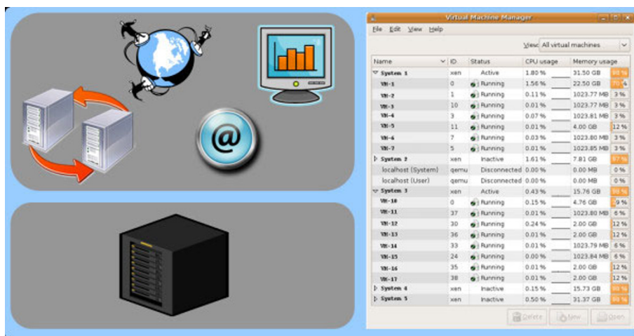
Figure 4 Server consolidation: A single powerful computer runs multiple virtual machines and serves as compute server, backup server and web server. Such a setup improves maintenance efficiency and reduces hardware costs. The right picture shows a production server with a XEN Virtual Machine Monitor and 17 independent running systems (Actual VM names were replaced; Picture source: Zhi-Wei Lu; UC Davis Genome Center Bioinformatics Core).
